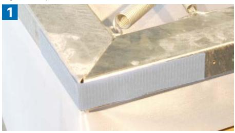
Attach the Velcro around the upper side of the frame with approx. 10 mm clearance from the outside (fig. 2 and 3).
