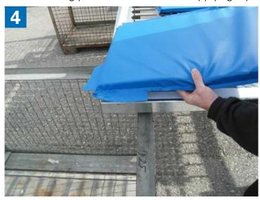
Position the short pad to line up and also apply light pressure to fix it to the frame. (Fig. 5)
