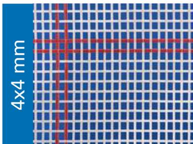
This jumping bed is made of 4 mm and 4 mm wide woven nylon bands sewn lengthwise and crosswise respectively. It offers the maximum permissible jumping performance according to FIG rules and is used in almost all trampoline competitions worldwide.
